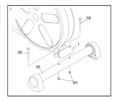
2. Attach the Front Stabilizer (3) to the Frame (1) with two M10 x 77mm Carriage Bolts (58) and two M10 Nylon Locknuts (84).
